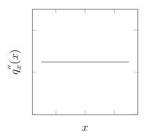
$T_1 < T_2$ . Since cross-sectional area,  $k_A$ ,  $k_B$  and  $q''_x(x)$  are constants, and  $2k_A = k_B$ , then T(x) from 0 to L/2 will have half the slope of T(x) from L/2 to L.
